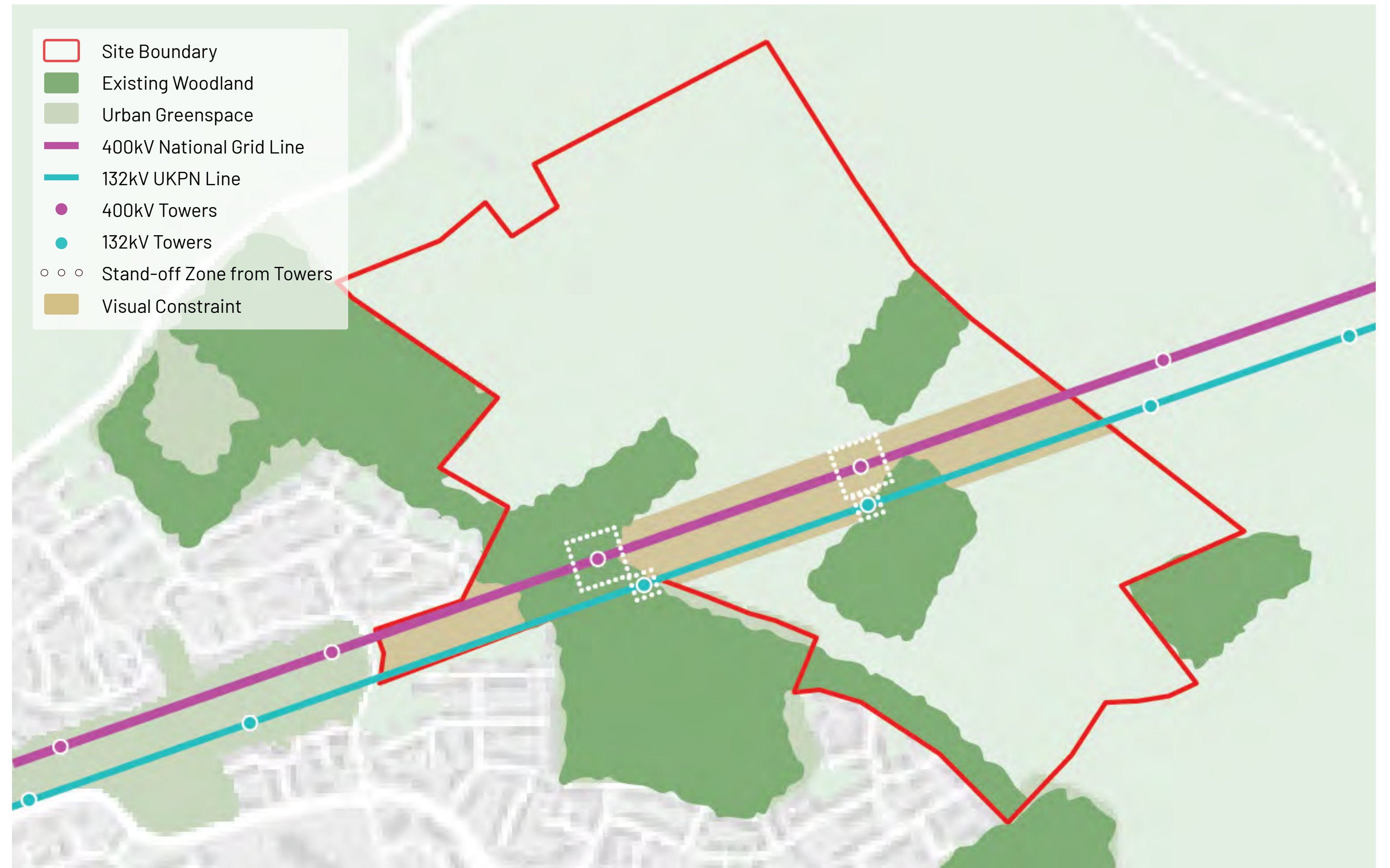
▲ Figure 9.1 - Utilities on the Site
